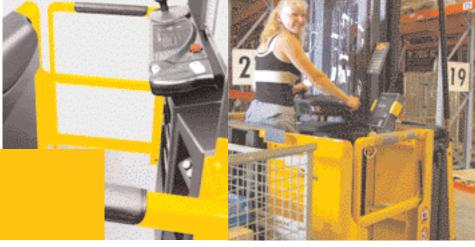
**OM-PIMESPO XOP3 vertical pickers** are compact, powerful vehicles and are capable of picking up to 10,480 mm.
